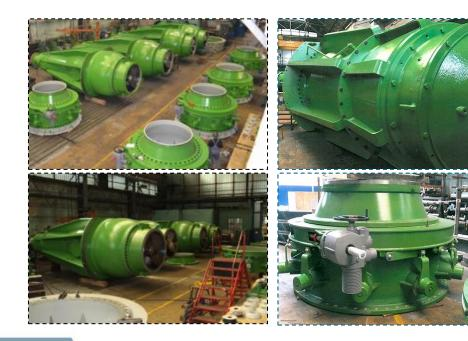
Axial and mix-flow one-stage semi submercible pumps equipped with control system hydro characteristic
